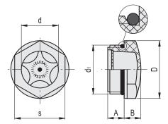
Code Description d1 А В D d 52 s HFTX.3/4-16 SAE 0.59 0.31 0.51 0.01 913691 3/4-16 UNF 1.02 0.87 HFTX.1 1/16-12 SAE 1 1/16-12 UNF 0.39 0.75 0.02 913731 0.59 1.38 1.18
